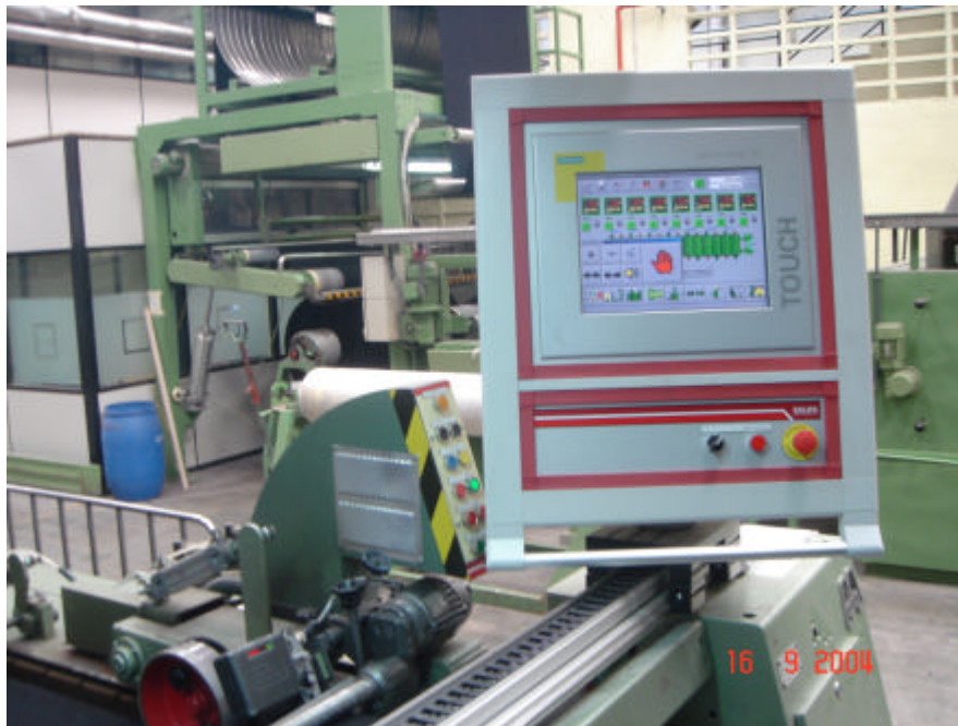
Main tactile screen with AUTORAME V1.0. control programme
